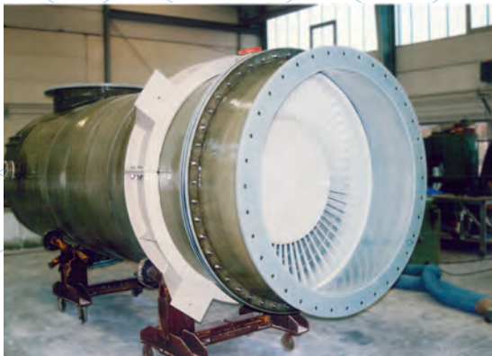
Swirl droplet separator made of PVDF/GFK in production
