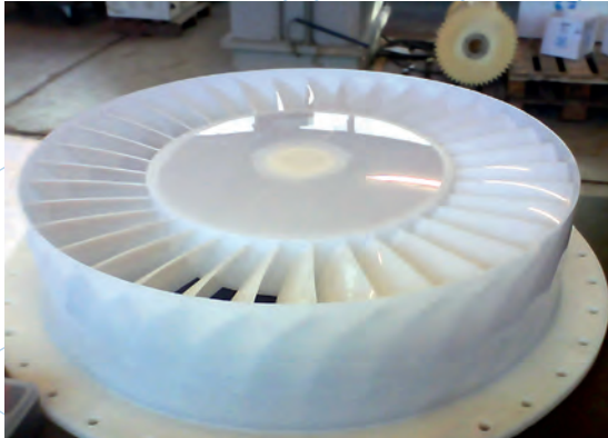
PVDF swirl generator in the workshop
