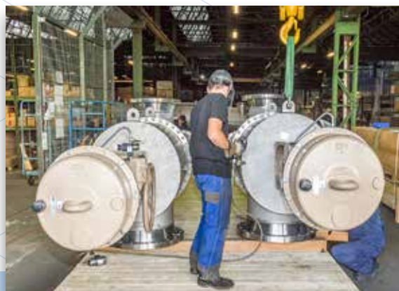
Thermocompressors in Körting Hannover AG's workshop
