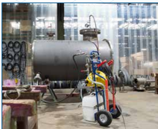
Hydrostatic tests up to 1 000 bar
