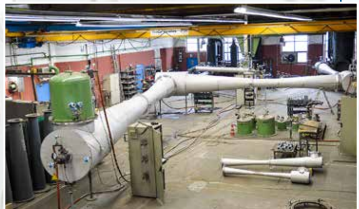
Performance test of three series connected steam jet vacuum ejectors with a suction pressure of 0.1 mbar
