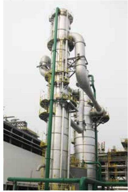
Bridge design, self-supporting (without separate steel construction), 2-tower design, 3-stage, countercurrent plant
