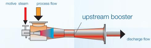
All systems are designed to operate with pre-condensers, but an additional booster can be installed upstream
