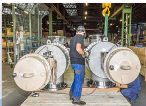
Thermocompressors in Körting Hannover AG's workshop
