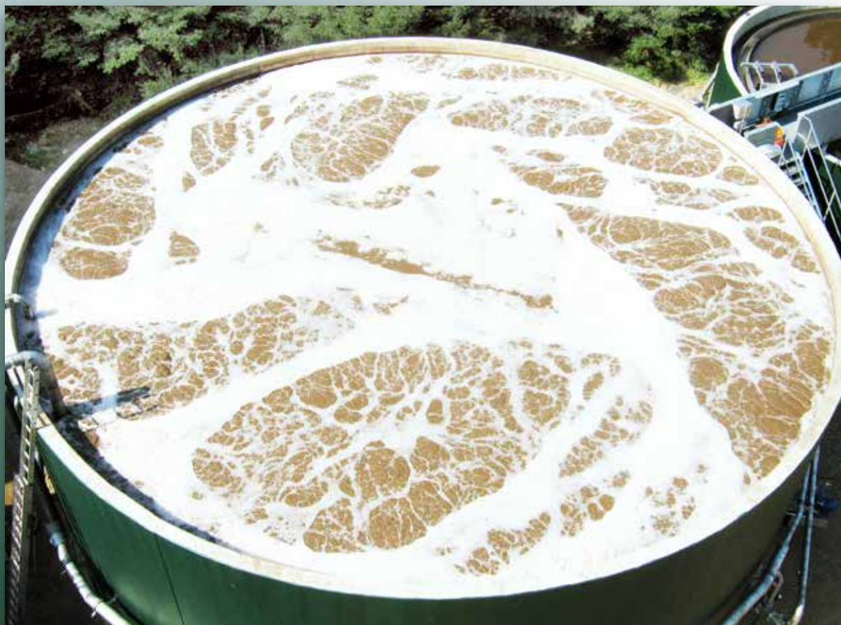
1 200 m 3 aeration tank for waste water from the paper industry
