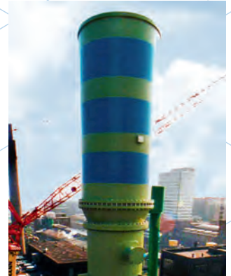
Chimney swirl droplet separator at Bayer
