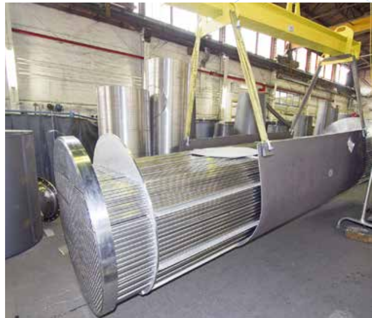
Assembly of a surface condenser destined for an oil refinery at the Körting plant in Hanover, Germany
